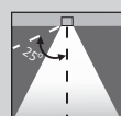
recessed lighting fixture with single-side vertically adjustable trim (for example 25°) and not rotatable horizontally
